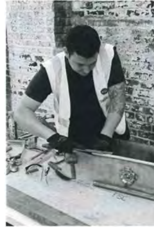
A Leadworker from Croft's demonstrates how to make a lead hopper head (above) and (below) a blacksmith from Ashmore Conservation makes a new wall plate
